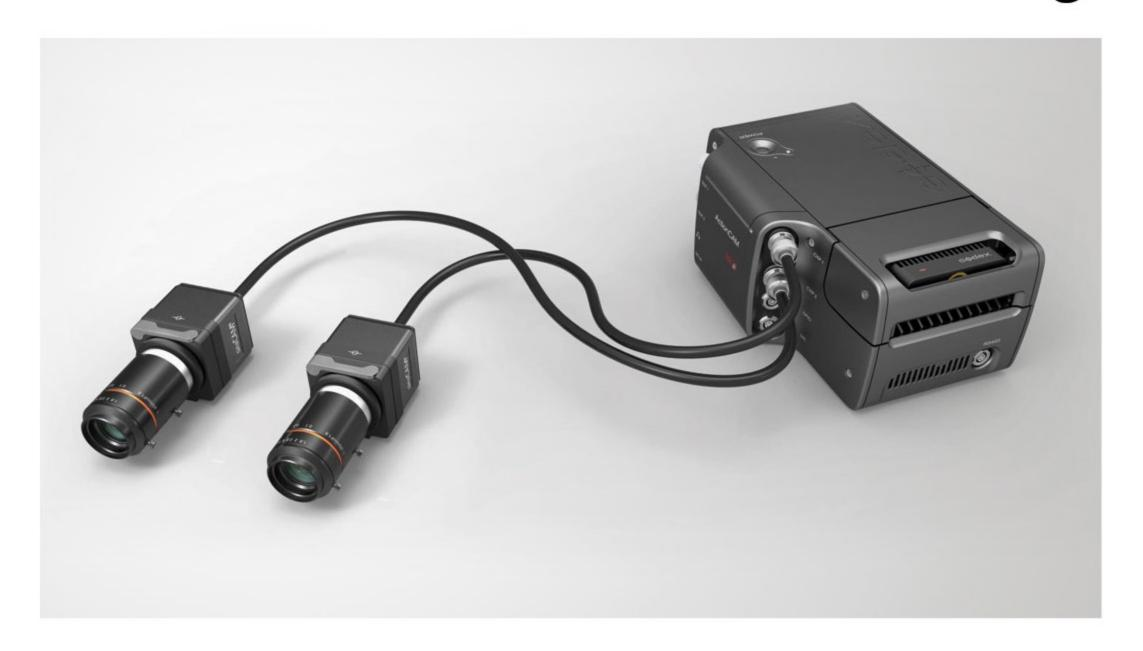
The Codex Action Cam consists of a RAW recorder and two special sinaCAM heads. It offers RGB, ProRes and Avid DNxHD output and additional sync compatibility.
